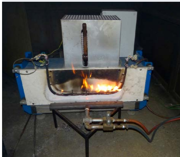
Fig. 4: Fire testing of the MegaLine® F6-90 S/F CI cables with resistance to fire, in accordance with EN 50289-4-16
