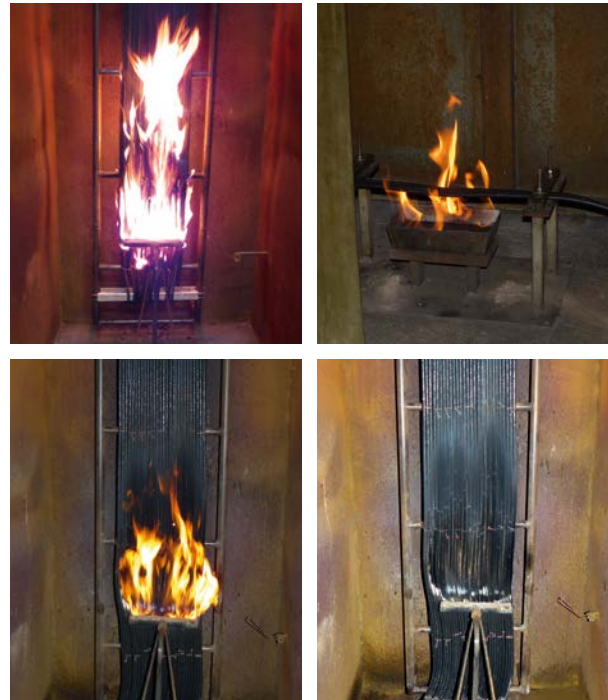
SeaLine® pursuant to EN 50399, Class B2 ca with max. burn-off length of 1.5 m
