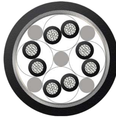
SeaLine® BWTS Cable 4x2x0.75 VZN BK Order no.: L45551-D42-K16
