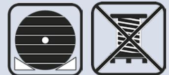
On pallets drums must be fixed in upright position
