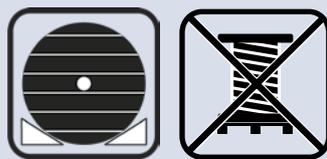
On pallets drums must be fixed in upright position
